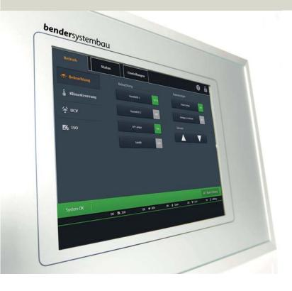
The built-in I/O system provides numerous options for embedding digital and analogue systems with various operating voltages, outputs, measurement signals and special functions within a single alarm indicator and operator panel.
