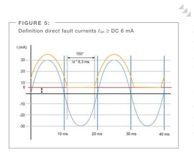
As a result of the joint discussions, the topic of monitoring DC fault currents  $I_{\Delta n} \ge DC$  6 mA arose. Residual current devices of type A in accordance with IEC 61008-1/IEC 61009-1 are only designed to trigger in case of sinusoidal or pulsating fault currents. In case of direct fault currents in the range  $I_{\Delta n} \ge DC$  6 mA, both the response time and the response value can be degraded on the usage of type A residual current devices (Figure 5).
