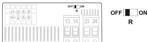
Activating a terminating resistor to define the first and the last device in the bus system.
