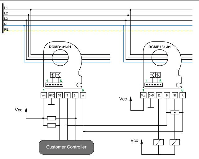
\* Terminating resistor 120  $\Omega$  must only be set on the last device in the RS-485 bus chain
