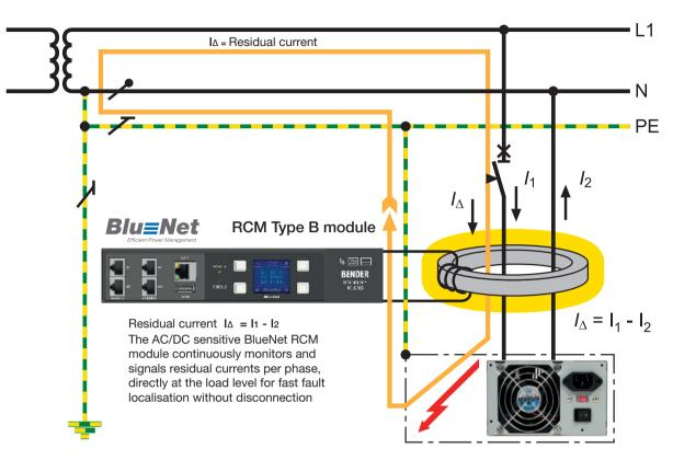
Residual current via the enclosure or the PE conductor in the event of damage, e.g. to a server power supply.
