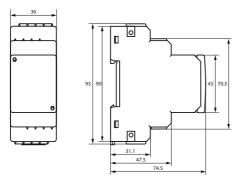
Figure: Dimension diagram (in mm)
