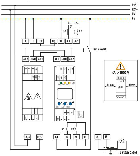
Figure: Wiring diagram with analogue interface
