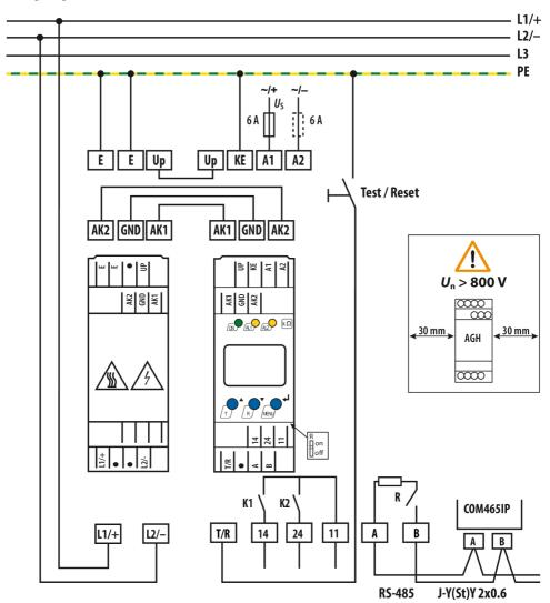
Figure: Wiring diagram with RS-485 interface
