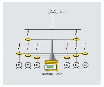
Bender's ground fault location systems find faults without shutting down
